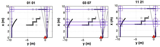
Fig. 6. A scene with detected features. Black points are raw measurements. Gray lines are those that were filtered. Blue lines are those who passed through the filter. Gray circles are all the real features, blue squares are those ones that were detected. Red triangle is the laser rangefinder location.
