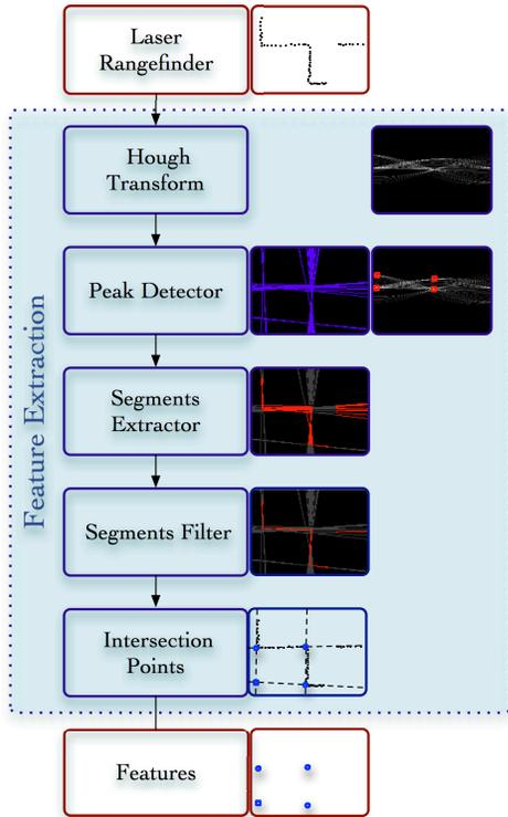
Fig. 2. Block diagram of the developed feature extraction algorithm.
